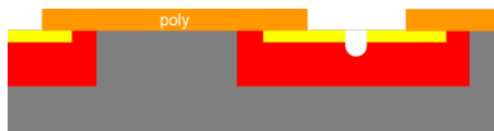
Figure 7. Schematic diagram after gate oxidation and deposition of polycrystalline silicon etching is completed.
