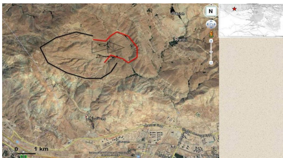
Figure 10. The Vardij landslide is located on the east side of Karaj region. The landslide was moved as a mass of crushed Eocene volcano sedimentary rocks of the Karaj Formation from the west to the east (ML1 in Figure 3).
