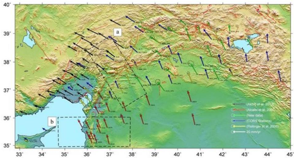
**Figure 8.** GPS measurements before the shocks of 6th February, 2023.
