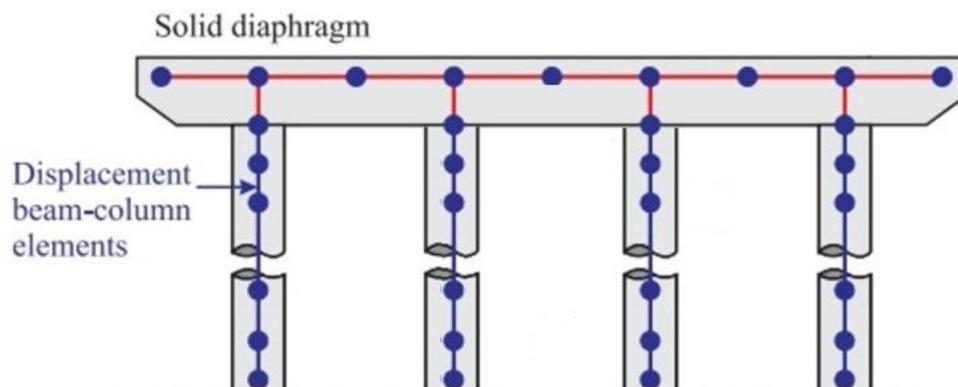
**Figure 1.** Cross-section (Elevation view) of the bridge.
