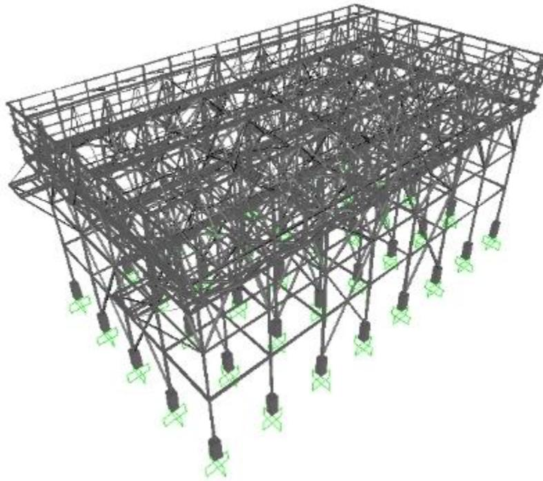
**Figure 6.** the steel ACC-model made in SAP for performing the elastic design.
