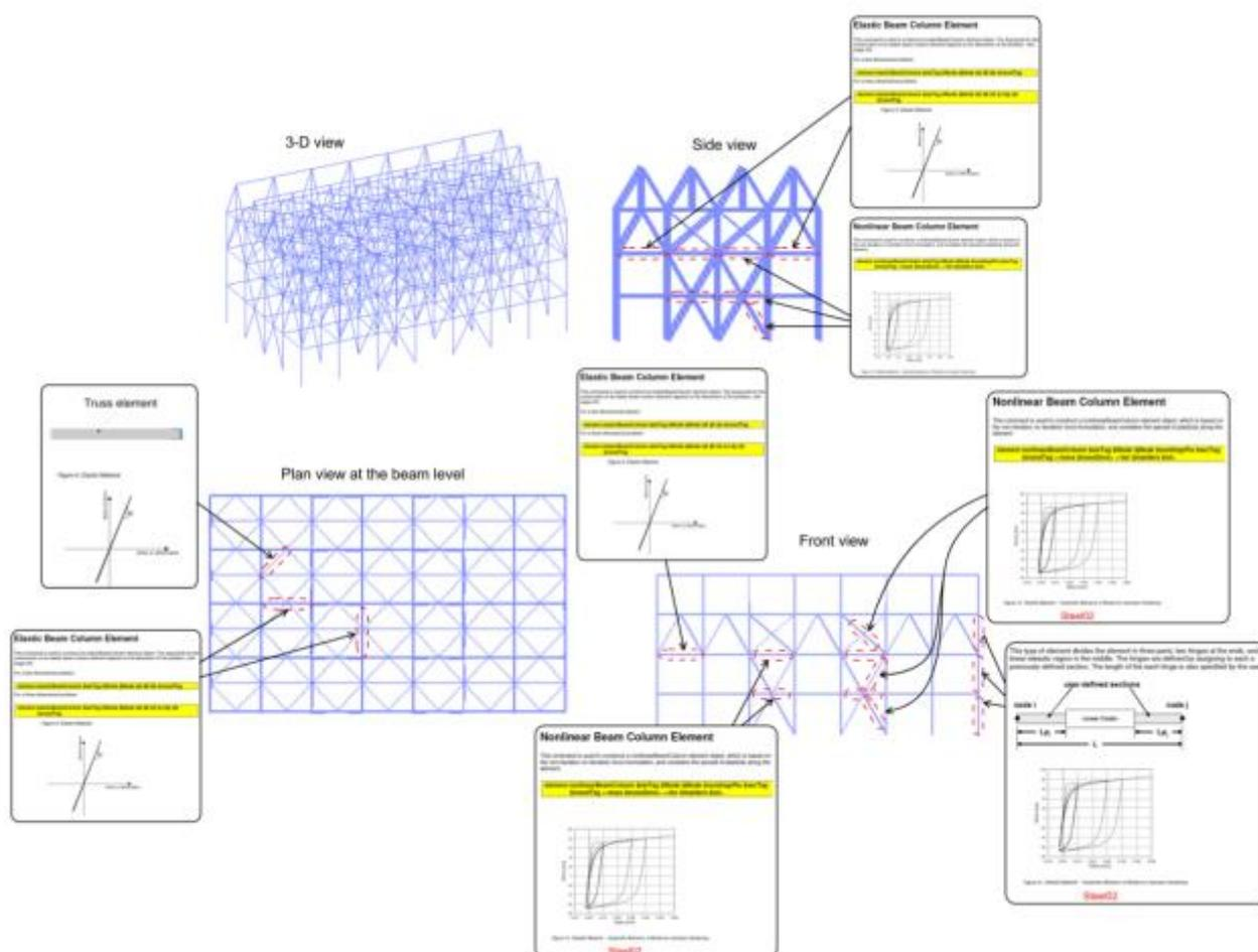
**Figure 3.** Structural elements and their mechanical properties in steel ACC model made in OpenSees.
