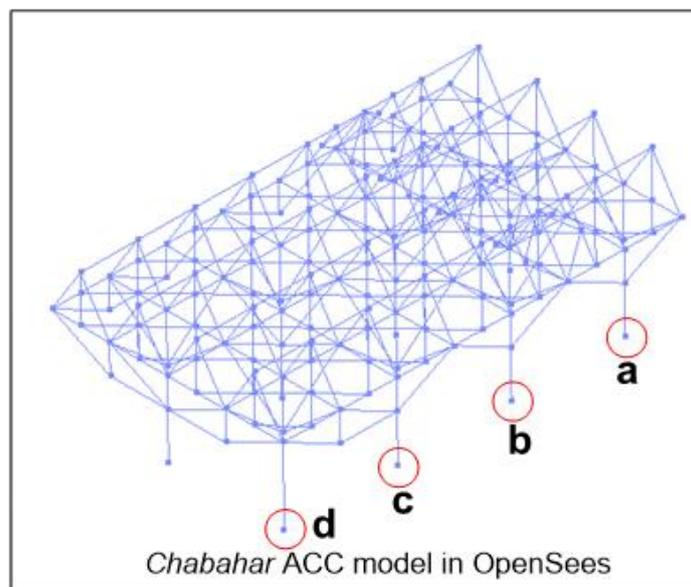
Figure 11. 3D model of Chābahār's ACC structure generated in OpenSees program.
