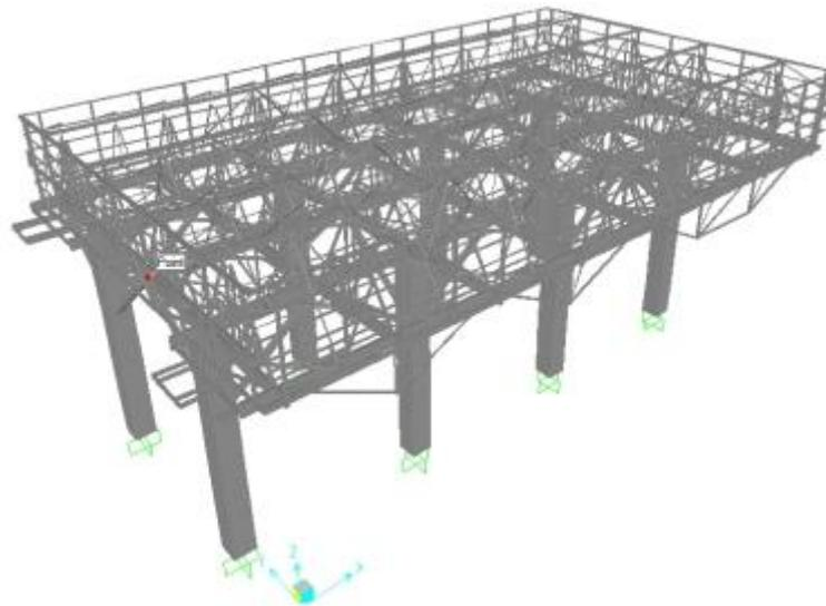
**Figure 10.** The concrete ACC-model in SAP software for conducting elastic design.
