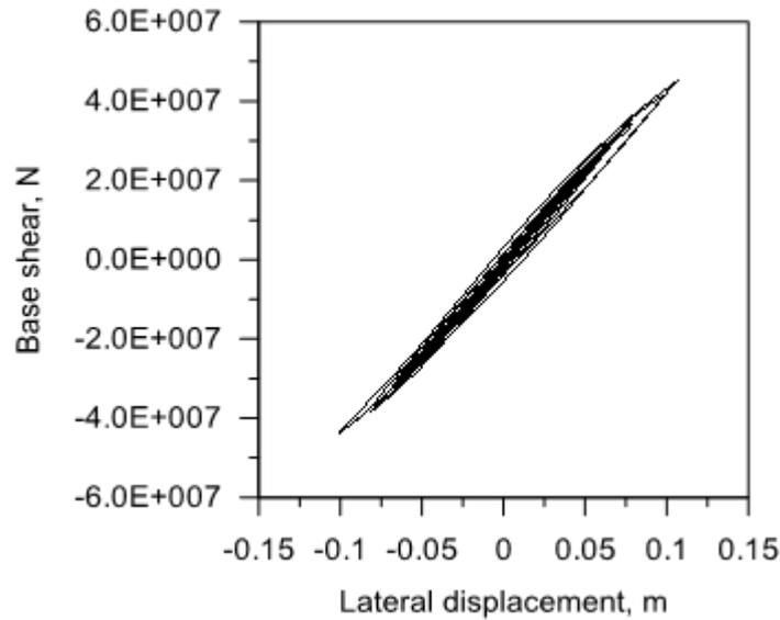
**Figure 9.** Base shear force vs. lateral displacement curve of Tous' ACC structure for earthquake in X-direction (displacement is measured at the roof level).
