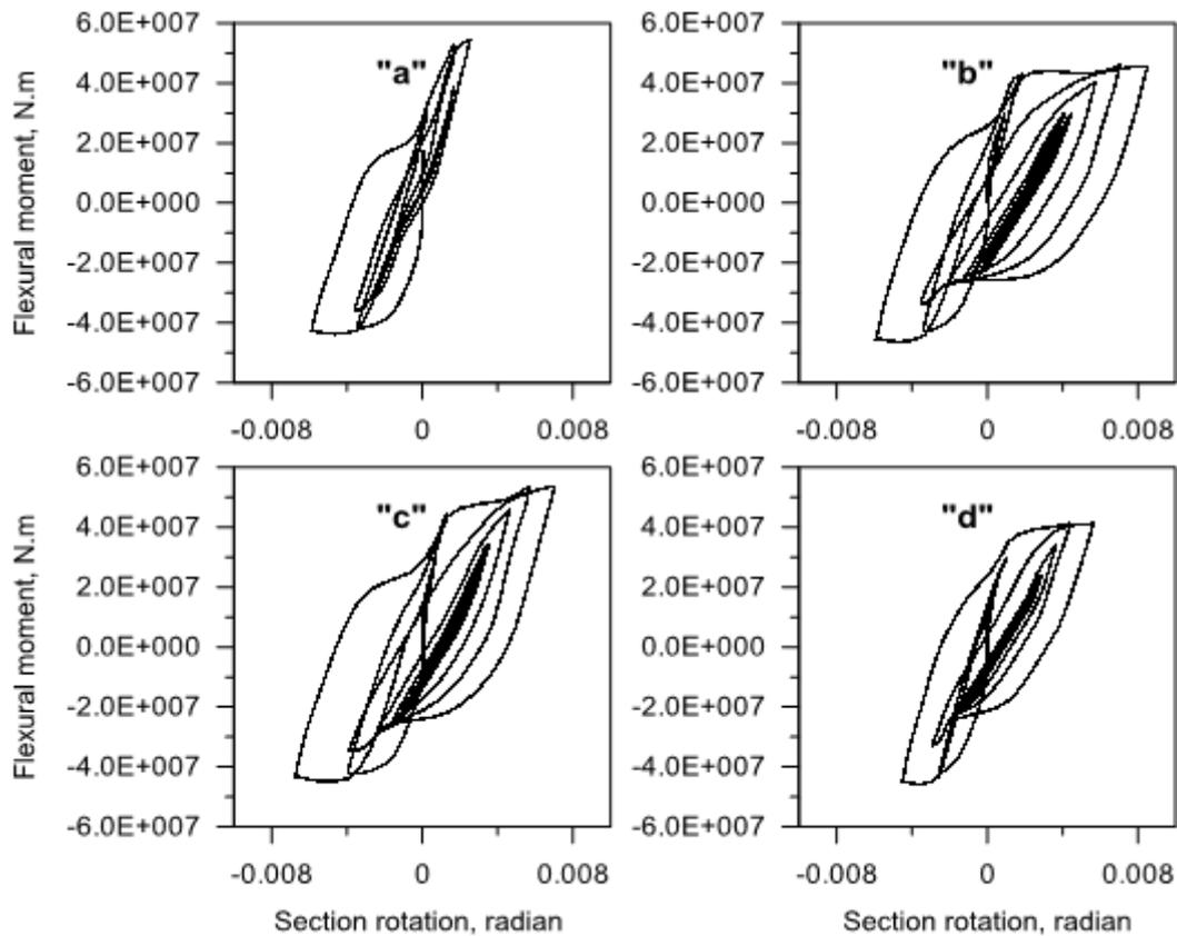
**Figure 12.** Moment vs. rotation curves of Chābahār's ACC columns at the column base.
