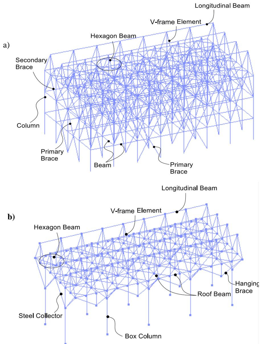
**Figure 2.** Various elements in the a) steel and b) concrete ACC model in OpenSees software.
