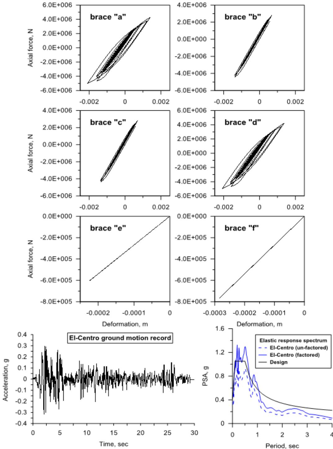
Figure 8. Axial force vs. deformation curves of Tous' ACC's various steel braces.
