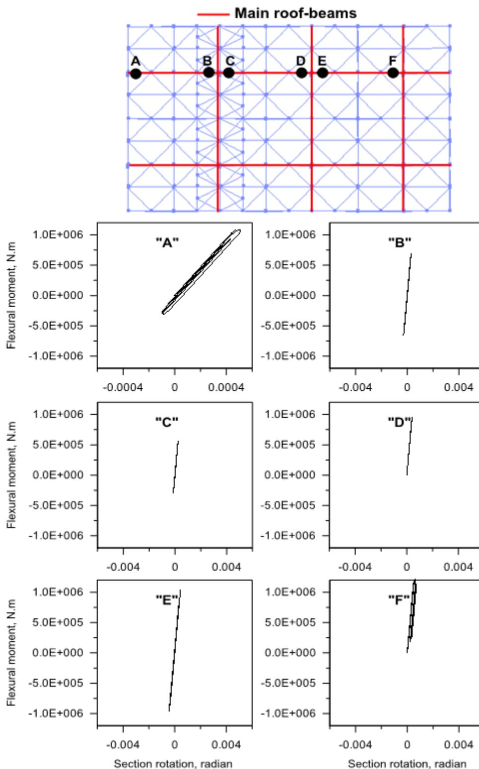
**Figure 13.** Moment vs. rotation curves of Chābahār's ACC roof beams.
