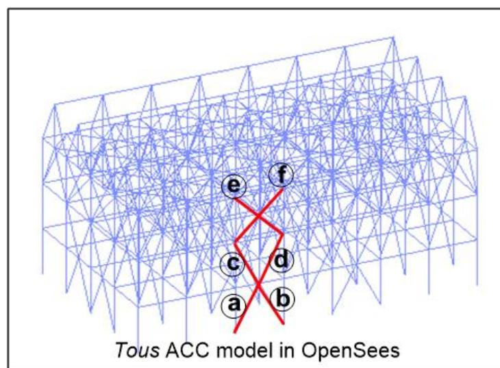
Figure 7. The 3D view of Tous’ steel ACC structural model in OpenSees program.
