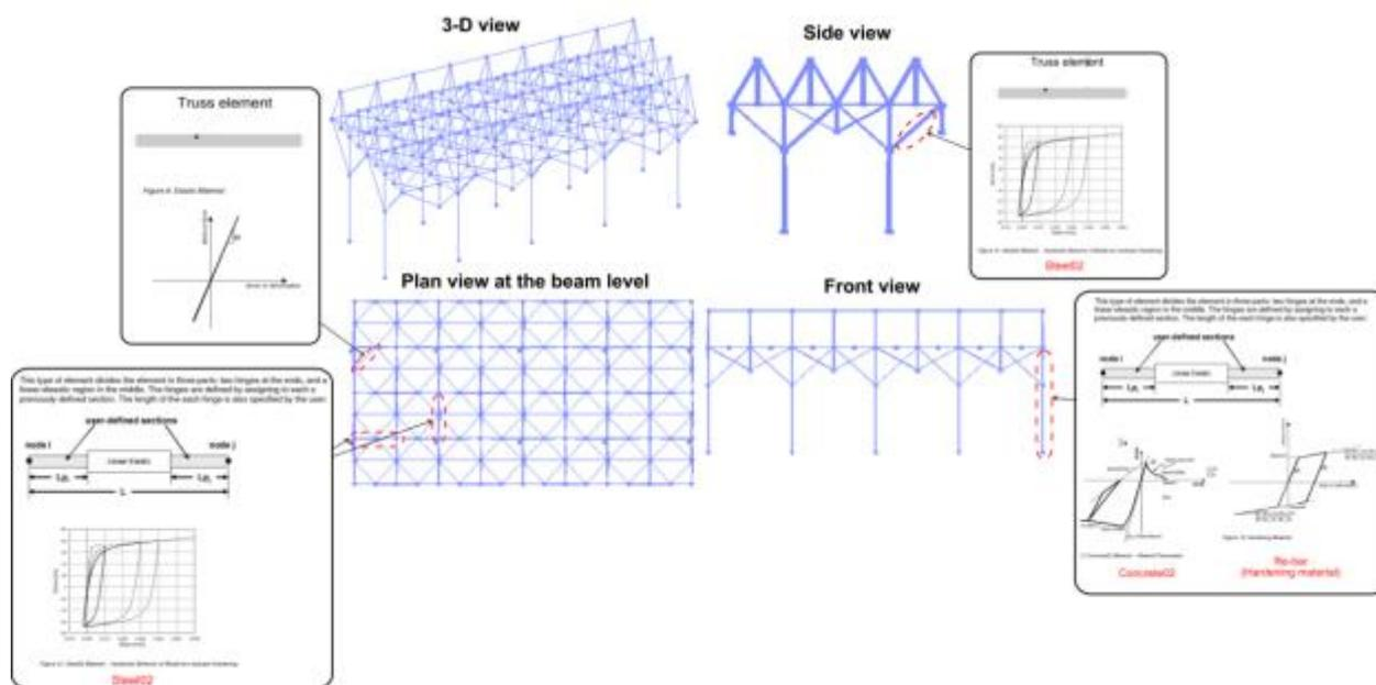
**Figure 4.** Structural elements and their allocated mechanical properties in OpenSees for the concrete ACC model.
