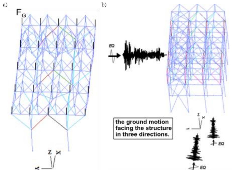
**Figure 5.** The ACC model subjected to a) gravity,  $F_G$  and b) earthquake loads.
