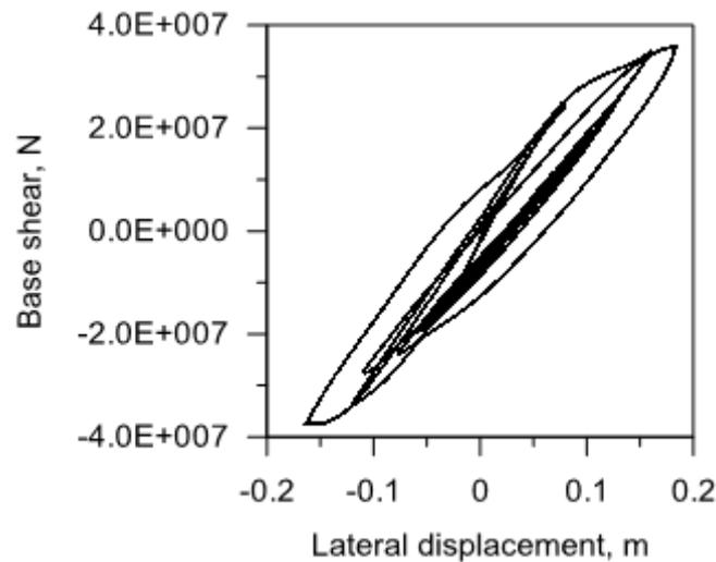
**Figure 14.** Base shear vs. lateral displacement curve for an earthquake in the X direction for Chābahār's ACC (displacement is measured at the roof level).
