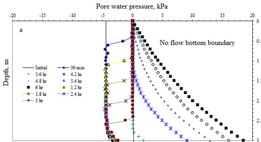
**Figure12(a)** Pore water pressure during rainfall intensity of 40 mm/hr. for both cases
