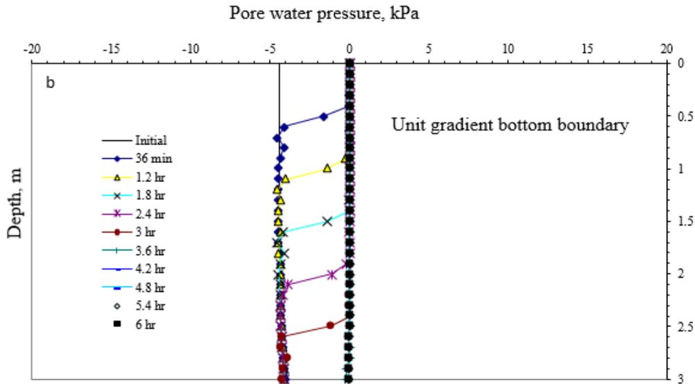
**Figure12(b)** Pore water pressure during rainfall intensity of 40 mm/hr. for both cases
