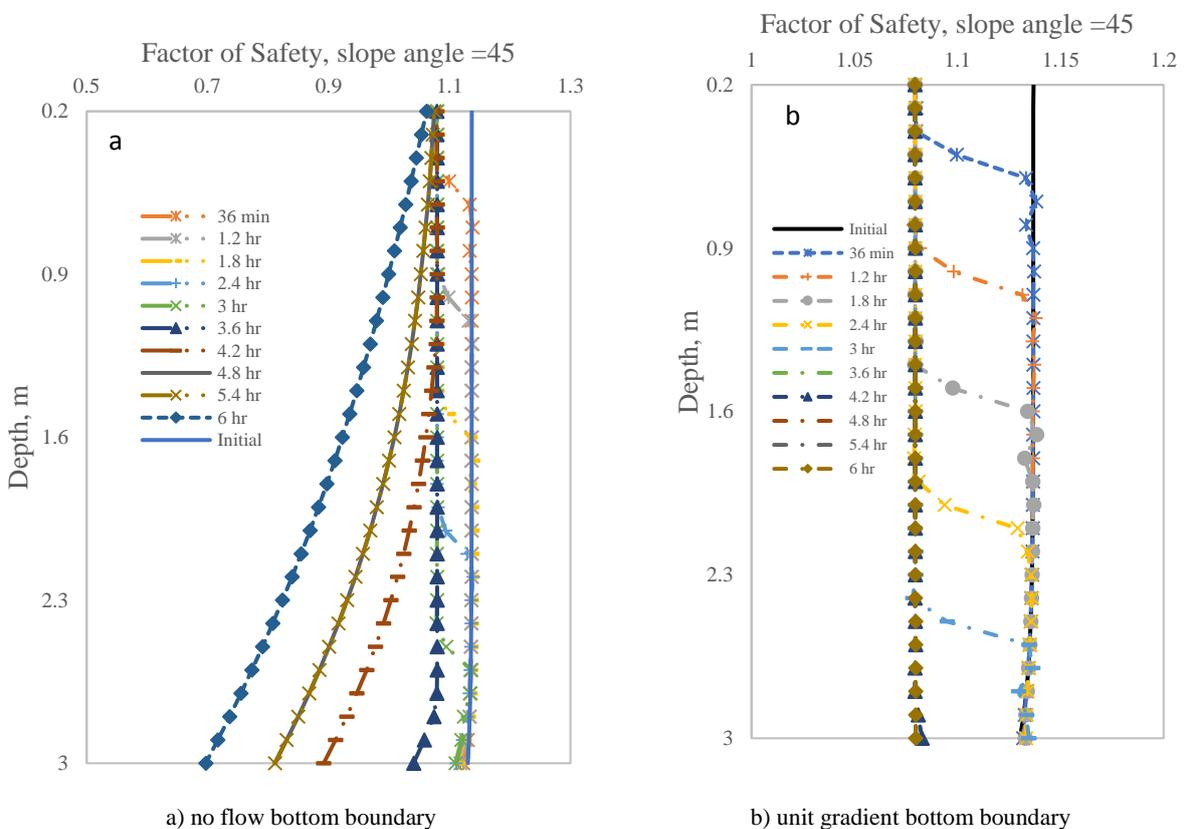
**Figure 13** Factor of safety during rainfall intensity of 40 mm/hr.
