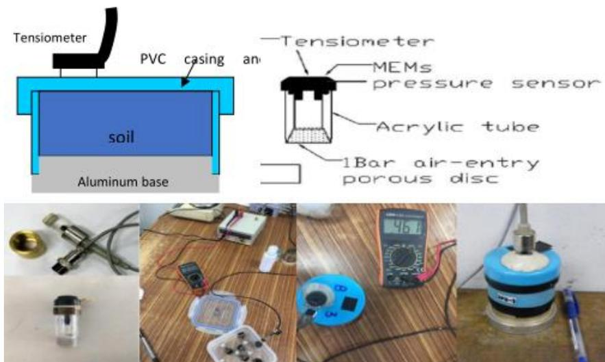
**Figure 6** The suction testing procedure and necessary equipment's
