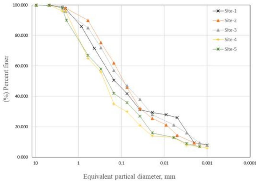
**Figure 9** The equivalent particle diameter and percent finer of collected soil curves
