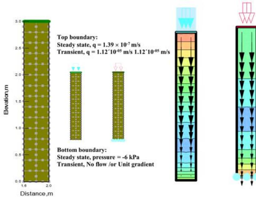
**Figure 11** Finite Element Mesh and result for the infiltration analysis for both case free draining and no flow boundary
