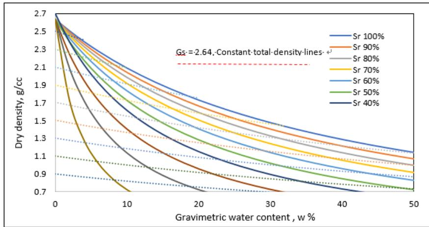
**Figure 8** Gravimetric water content versus dry density with constant total density for specific gravity
