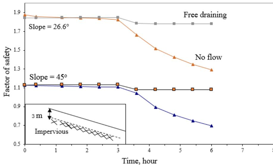
**Figure 14** Factor of safety during rainfall intensity of 40 mm/hr. a) no flow bottom boundary b) unit gradient bottom boundary
