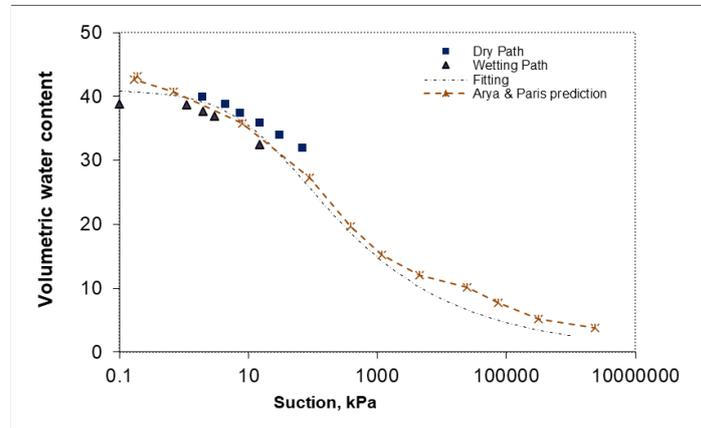
Figure 10 Soil-water characteristic shapes of soils from a landslide-prone area of Chittagong
