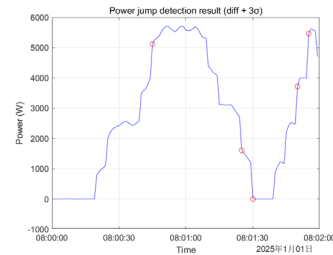
Figure 3. Power transition point detection based on differential threshold.
