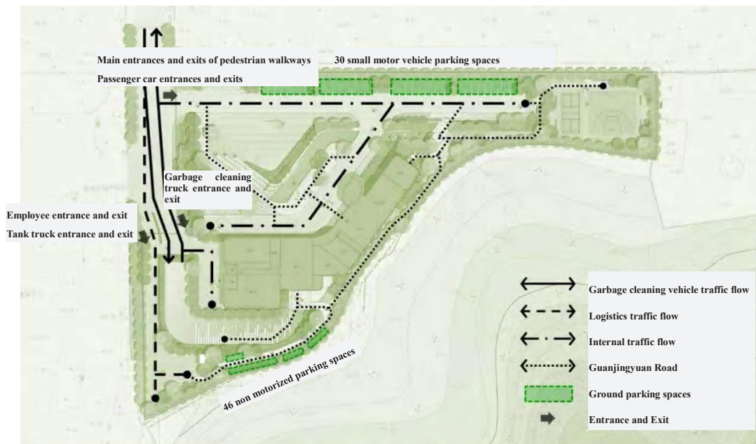
Figure 5. Schematic diagram of transportation and logistics organization at transfer stations.
