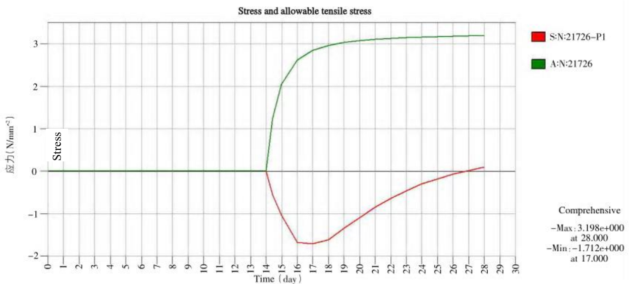
Figure 7. Maximum tensile stress point variation curve of the second layer of the pier cap.
