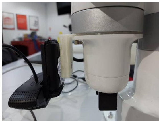
Figure 5 Installation of camera mounting plate on end-effector
