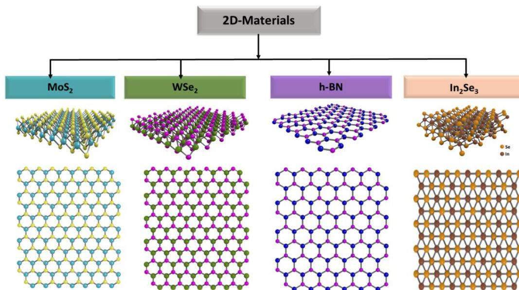
**Figure 1.** Schematic illustration of various 2D materials such as MoS<sub>2</sub>, WSe<sub>2</sub>, h-BN, and In<sub>2</sub>Se<sub>3</sub>.
