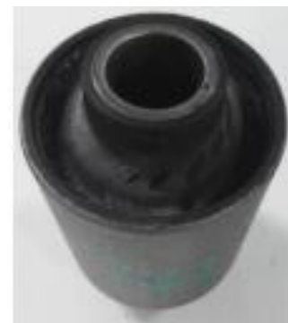
Figure 9. Bushing after bench fatigue test.
