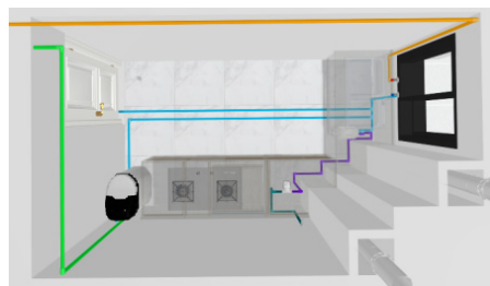
Figure 3. Kitchen waterway construction.
