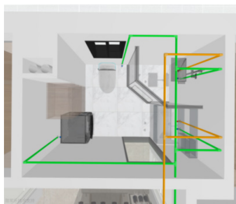
Figure 4. Toilet waterway construction.
